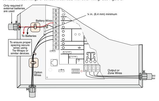
Figure 5: Non Power Limited Wiring
