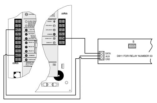
Figure 18b: D811 Module Wiring to the D7412G
