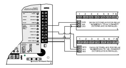
Figure 17a: D8129 Connections to the D9412G
