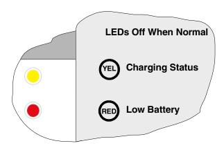
Figure 6: Charging and Battery LEDs
