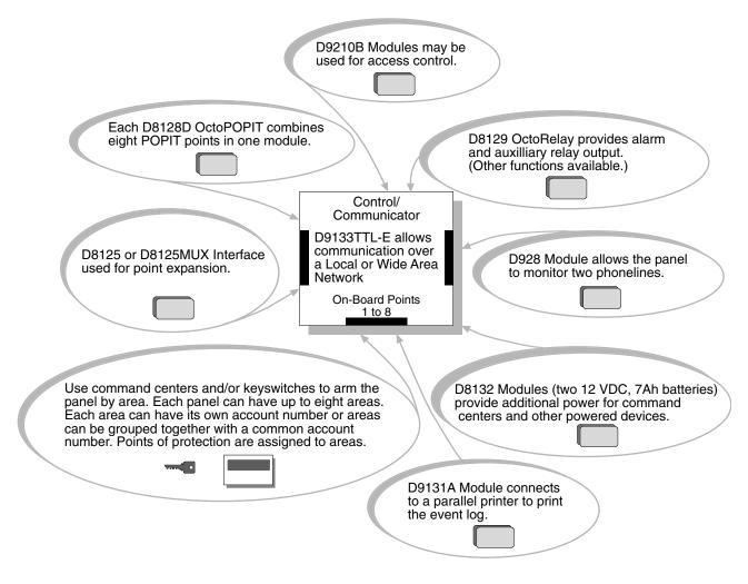
**Figure 1: System Configuration**
