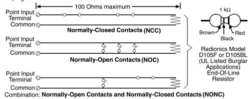
Figure 12: On-board Point Sensor Loop Wiring
