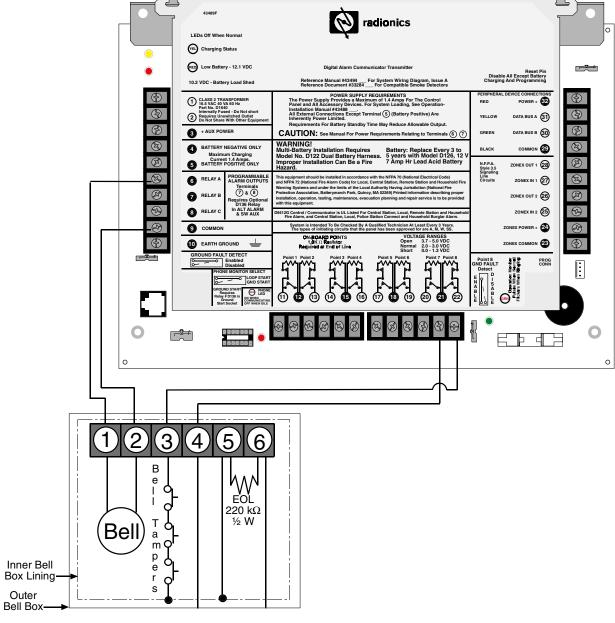
Figure 13: Wiring for Installations using the Ademco AB-12 Bell/Housing
