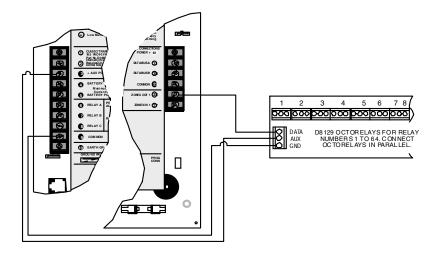
Figure 17b: D8129 Connections to the D7412G
