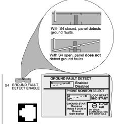
Figure 3: Ground Fault Detect
