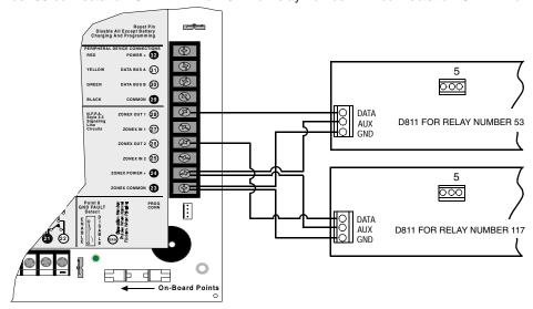
Figure 18a: D811 Module Wiring to the D9412G
