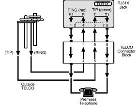
Figure 8: RJ31X Wiring
