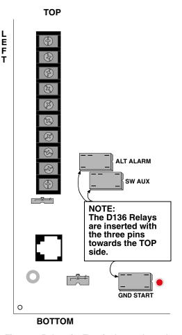
Figure 7: Relays for Terminals 7 and 8 and Ground Start
