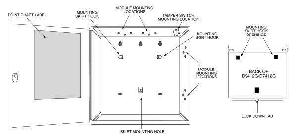
**Figure 2: Enclosure Mounting**
